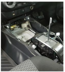
Remove the gear stick by unscrewing it counter clockwise
