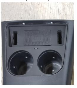
9. Once the charger is mounted and tested, clip in the side bumpers
