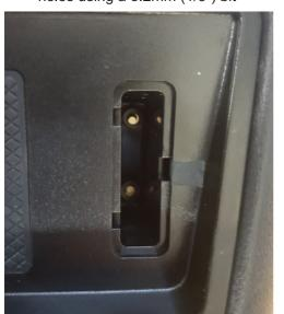
5. Slide the retaining clip into place and clip charging panel to center console
