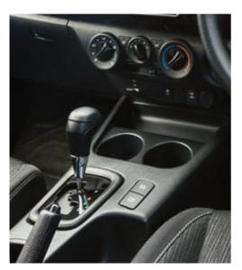
2. Remove the center console complete trim by unclipping it directly up
