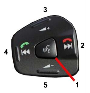
Single Press (Button 1) switches display on Press & Hold Speech Button (button 1) for 2 seconds this will enable menu mode option.
