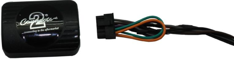
3. Connect the opposite end of head unit patch lead to the head unit steering wheel control input on the back of the aftermarket head unit. This may be a 3.5mm jack plug or a wire input depending upon the head unit brand being fitted. Please see the head unit installation manual for further information on where to connect.
