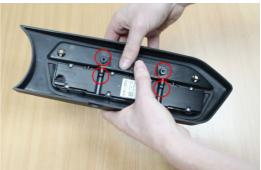
**15.** Place the button panel assembly in front of the display screen. Screw the panel into place – Screws highlighted in the picture, then push the rubber mat into position.
