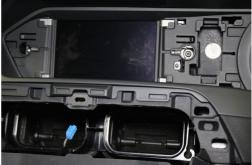
**7.** Fascia assembly: Screw the radio fascia brackets onto both sides of the fascia panel supplied in the kit. (2x screws each side - ITEM 7)
