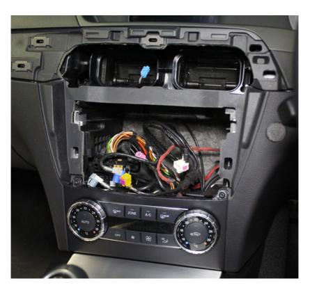
**6.** To remove the display panels (each side) push the panels inwards towards the display screen.
