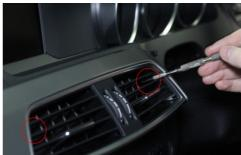
2. When removing the air vent panel make sure you unplug the blue connector to the air vent controls.
