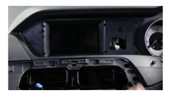
**12.** On the OEM head unit unscrew the four screws on the bottom of the button panel and remove the button panel.
