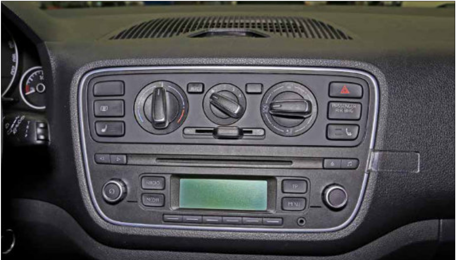
OEM dashboard SEAT Mii / SKODA CITIGO / VW up! with manual air conditioning
