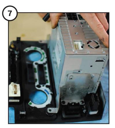
Attach the double DIN stereo to the mounting brackets and main fascia panel, and screw into place.
