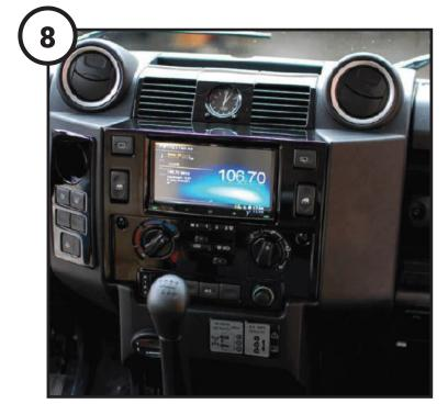
Place the stereo into the dashboard and make all wiring connections to the stereo. Reassemble the remaining dash components in the reverse order of
