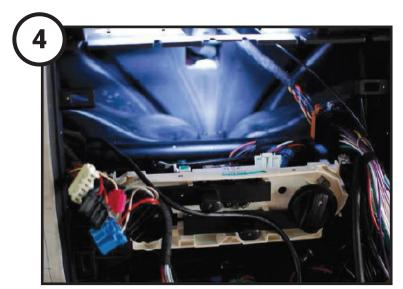
Remove the metal clips and reroute the air vent wiring
