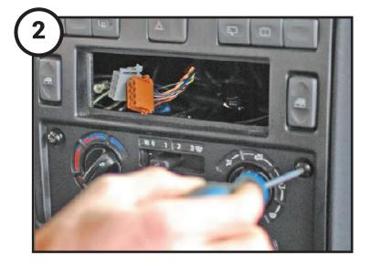
Remove the T-30 screws from the main OEM fascia panel
