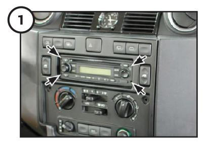
Remove the OEM radio using a set of release keys
