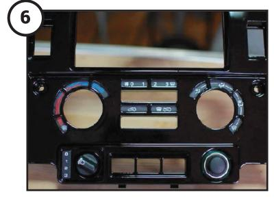
Install the buttons/switches previously removed from the OEM fascia panel into the new fascia panel. Make sure that the cluster detail is also pushed into the fascia panel
