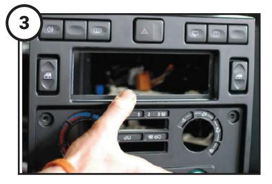
Remove the fascia panel and all buttons/switches, including the OEM clock
