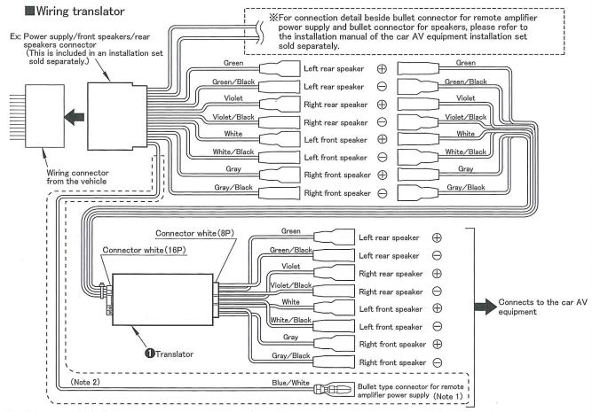
Note1.Connect the bullet type connector from the car AV equipment remote amplifier power supply so that the Factory amplifier and Factory speaker system can be used. If the car AV equipment does not use the remote amplifier power supply, insert ACC power. If not inserted, sound will not issue.
